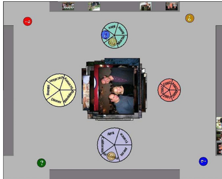
Fig. 5. The TeamSearch UI with parallel query tokens. The blue user and the yellow user have created two separate queries (location = “Sri Lanka” and people = “Lisa” in yellow; people = “Larry” in blue), and each sees the results for his own query in his own results tray. (For interpretation of the references to color in this figure legend, the reader is referred to the web version of this article.)
