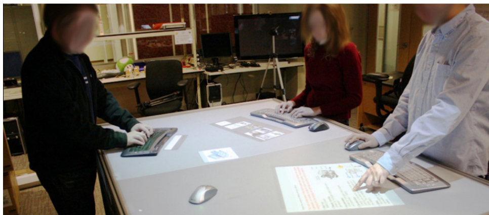
Fig. 6. A group gathers around FourBySix, a large, standing-height tabletop that supports mouse and keyboard input, to conduct a collaborative search task.
